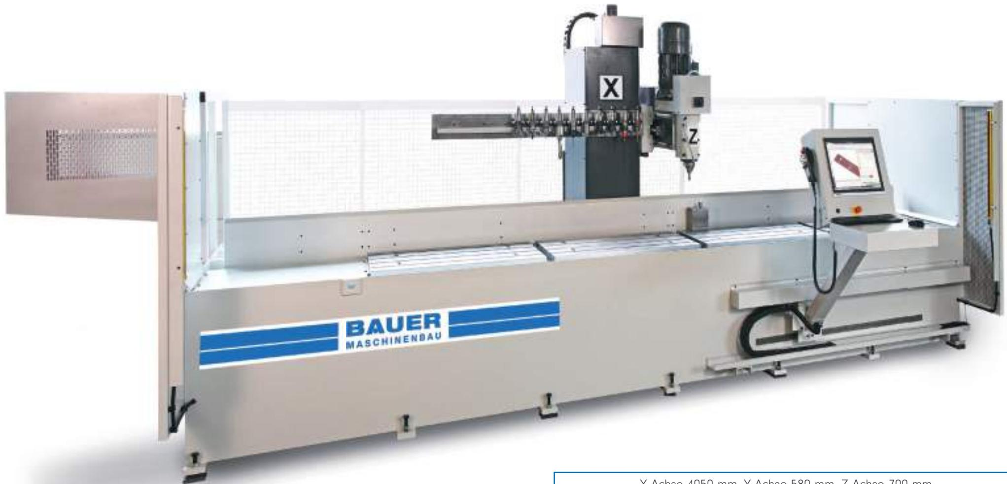
X Achse 4050 mm, Y Achse 580 mm, Z Achse 700 mm
